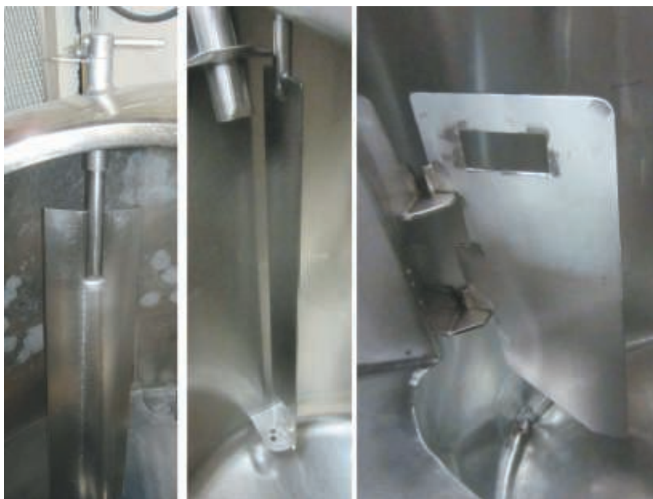
FIGURE 1. These three types of baffles can be adjusted while the tank is filled
