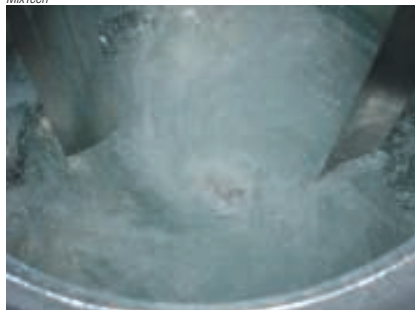
FIGURE 7. A deep vortex can be created by bottom-mounted high-shear dispersers
