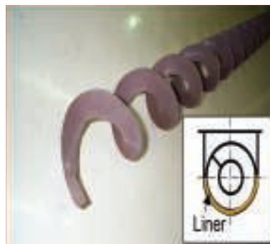
FIGURE 3. The flights on a shaftless, screw-type conveyor have robust construction, which allows them to resist damage by torsional wind-up
