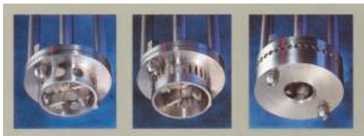
FIGURE 9. Some rotor-stator dispersers have an impeller with blades rotating inside a stator with slots or holes
