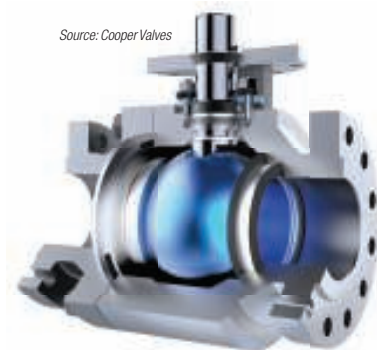
Source: Cooper Valves FIGURE 4. Accuseal metal-seated ball valves offer Omni-Lap 360, which mate-laps the entire ball and seat for optimal roundness, producing 100% ball-to-seat contact
