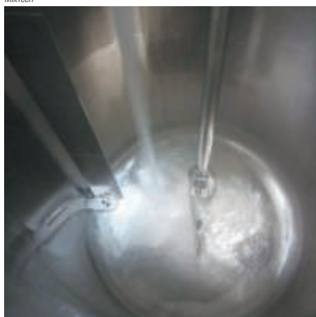
FIGURE 3. This rotary-head disperser is mounted offset from the center
