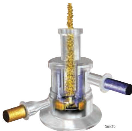
FIGURE 13. Some inline dispersers add powders to liquid
