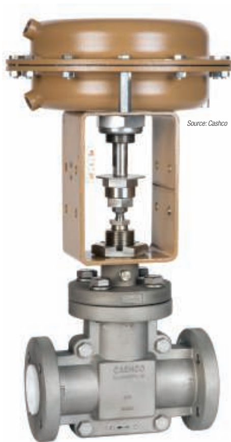
FIGURE 1. Model 521 is a sliding stem, globe-style, bellows-sealed, pneumatically actuated control valve designed for maximum corrosion resistance in pure chemical service
